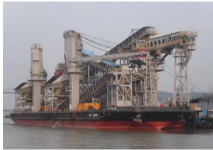
The FLF Ratu Barito which can load up to Cape size vessels at rates of 40,000 tonnes per day
