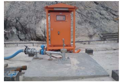
Slope dewatering continues to be a priority to ensure slope stability within the Tutupan mine
