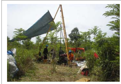
Reserve definition drilling in progress at Wara
